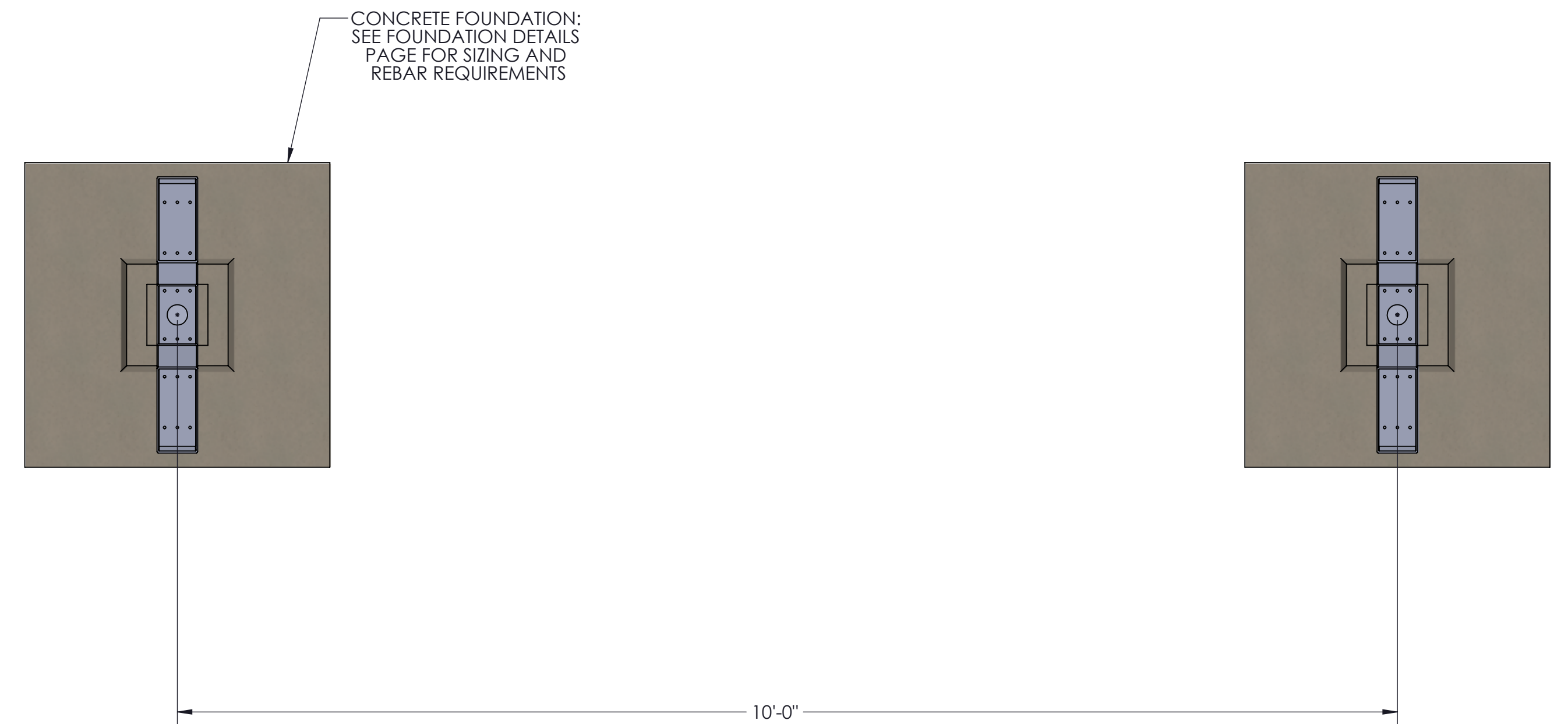
TOP VIEW FOOTING LAYOUT
